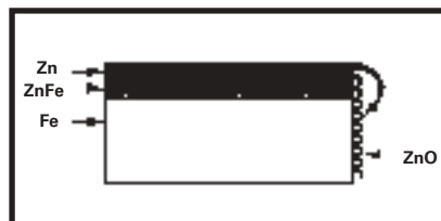
Protection of cut edges with zinc coatings.
