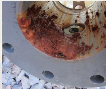
In these images taken 14 months after installation you can see many of the tubercles common to MIC and extensive corrosion.
