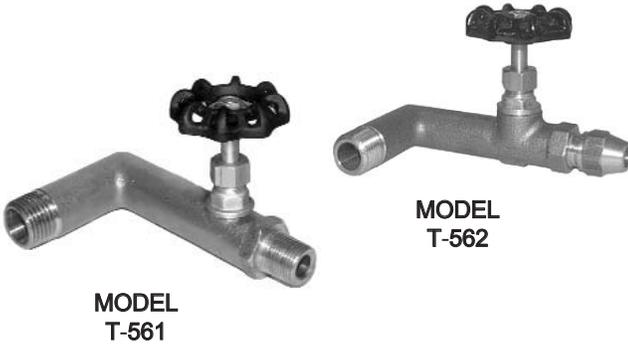
**LEGEND MODEL T-561/T-562** oil tank valves are constructed of heavy duty brass. They have a screwed bonnet, rising stem, and metal-to-metal seat. Designed for use as a bottom supply shut-off valve.
