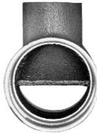
**LEGEND MODEL T-569** venturi tees and **MODEL T-570** mono-flow tees are constructed of cast bronze. The T-570 is a scoop design while T-569 is a venturi design.
