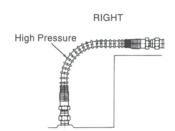
Avoid a sharp twist or bend in the hose by using the proper angle adaptors.
