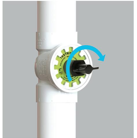
4 Open stem by turning counter-clockwise. Drain system completely. Remove Test Wedge.\*\*\*
