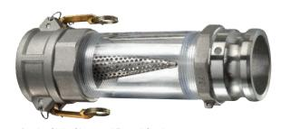
The pictures above show a popular installation set up for the Sight Glass and Funnel Strainer. The picture on the left shows the Funnel Strainer assembled with an aluminum type "D" coupling. The picture on the right shows the complete assembly with the Sight Glass and an aluminum type "A" coupling. Warning: Never use a wrench on the Sight Glass - always tighten the connecting pieces.
