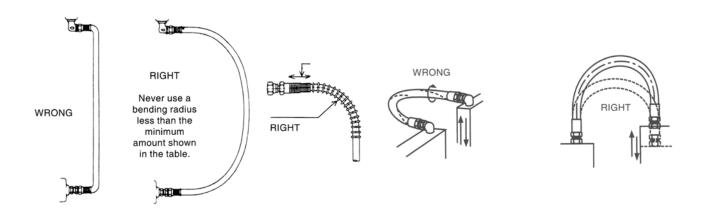
To prevent twisting and distortion, hose should be bent in the same plane as the motion of the boss to which the hose is connected. Never use a bending radius less than the minimum shown in the hose specification tables. Avoid sharp bends in hoses to reduce collapsing of lines and restriction of flow by using a proper spring guard. Exceeding minimum bend radius will greatly reduce hose assembly life.
