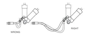
Where the radius falls below the required minimum, an angle adapter should be used as shown above to avoid a sharp bend in the hose.
