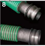
Step 8 — Insert the coupler's barbed shank into the hose, twisting counterclockwise for TDH, TV, TVHD, and VAPR and clockwise for NDH as it enters. For ease of installation, an appropriate lubricant may be used.
