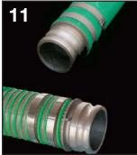
Step 11 — Install two hose clamps over the hose end above the coupling. When using banding coils, be sure to tighten clamps in a clockwise direction for TDH, TV, TVHD, and VAPR, and a counter-clockwise direction for NDH, so the banding coils tighten down on the hose.
