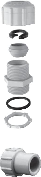
Kraloy's Nonmetallic Strain Relief Connectors are supplied with all the components you need for a complete connection. The connector body, a selection of grommets and compression rings accepting a range of cord dimensions, a sealing 'O' ring and metallic locknut are all supplied in one package. Available in 1/2" and 3/4" threaded hub and 3/4" PVC socket solvent weld configurations to accommodate a variety of applications.
