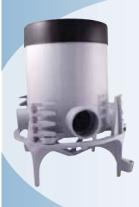
This simple yet innovative Round Floor Box Stand is equipped with several height brackets which accommodate the different rebar and post-tension cable heights and slab depths found from job-site to jobsite. When installed together, the Floor Box and Stand can be used in 5-1/2" to 10" slab depths.
