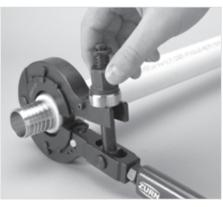
the tool jaws. Confirm the tool is at a 90° angle to the fitting and close jaw. Hand tighten the nut to hold fitting assembly in place.
