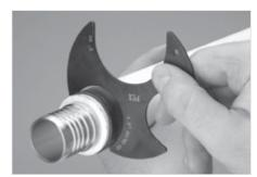
Checking Check crimp using the supplied gauge.
