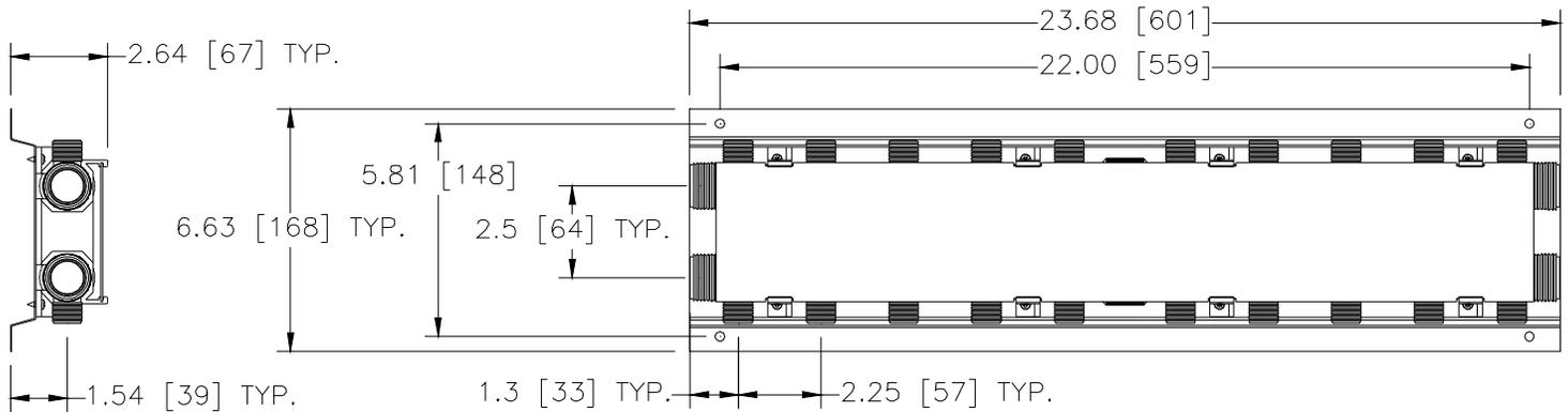
**Engineering Specification:** ZurnPEX® 1" diameter polysulfone QickPort® Pre-Assembled Manifold comprised of ten (10) hot and ten (10) cold 1/2" male straight pipe thread outlets and four (4) 1" male pipe straight thread inlets. Manifold is rated at a maximum pressure of 100 PSI at 180°F. Optional shut off valves can be added for individual on/off control of each distribution line. NSF listed. For use with potable water only.
