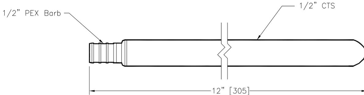
**Engineering Specification:** ZurnPEX® 1/2" Straight Copper StubOut. 1/2" PEX Barb x 1/2" CTS. End spun closed allows for system testing before valves or other fittings are installed. Meets NSF® and ASTM requirements.
