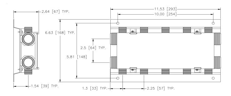
**Engineering Specification:** ZurnPEX® 1" diameter polysulfone QickPort® Preassembled 5 x 5 Manifold. Comprised of five (5) hot and five (5) cold 1/2" male straight pipe thread outlets and four (4) 1" male pipe straight thread inlets. Manifold is rated at a maximum pressure of 100 PSI at 73°F with valves, and a maximum pressure of 160 PSI at 73°F without valves. Optional shut off valves can be added for individual on/off control of each distribution line. NSF listed.
