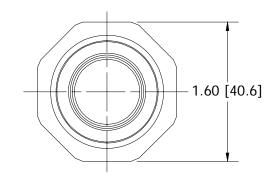
**Engineering Specification:** The Zurn PEX<sup>®</sup> Plastic Manifold 1" x 1" Coupling. Made from Acetal. The QC55FQP is used to link components together to expand QickPort<sup>®</sup> manifolds. Meets requirements of NSF-61.
