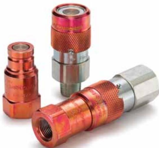
FH Series high pressure, non-spill couplings have flush valves and are designed to minimize spillage and air inclusion when connecting or disconnecting. Couplers and nipples are steel with nitrile seals. Available in 3/8 inch size only, with red finish for easy identification. Will not connect with lower pressure flush face couplings.
