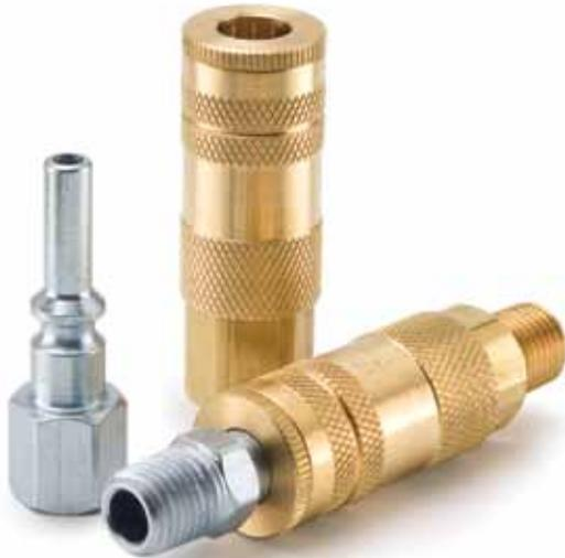
70 Series Pneumatic Couplers are interchangeable with Lincoln's "Long Stem" series couplings. Couplers have brass bodies and steel valves. Nipples are constructed of steel. Sleeve-Lok is an optional feature.
