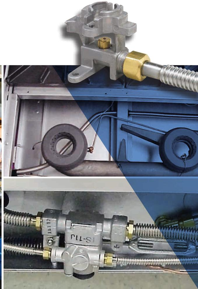
**F**lexTube Replacement Installation Kits have been specifically designed to replace damaged internal supply lines on commercial cooking equipment. These kits are to be used as replacement components for rigid aluminum tubing. FlexTube corrugated stainless steel tubing will minimize the time spent to replace these fuel lines.
