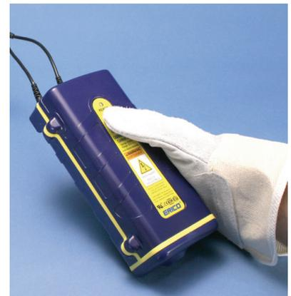
**STEP 4** Press and hold operate button. Open mold after 10 seconds.
