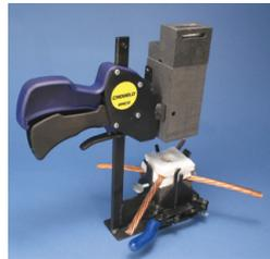
**STEP 1** Layer batting and variable conductor sizes to be welded into dry mold.
