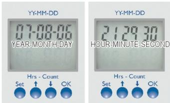
3. When time/date is set an option for CLEARING ALL DATA appears. Select option Yes or No with UP and DOWN arrows and confirm it by pressing OK. WARNING! Once data is cleared it can't be retrieved.
