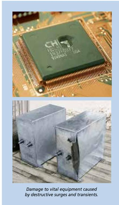
*Damage to vital equipment caused by destructive surges and transients.*
