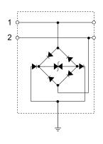
The MWERJ451 and MWERJ452 series of broadband wireless surge protection products are designed to provide economical and reliable protection from lightning and other transients. Part of the ERICO line of facility electrical protection products, the MWERJ451 and MWERJ452 are enclosed in a weatherproof enclosure for protection in harsh environments. They can be easily mounted on a flat surface or pole. The products connect to the service in a pass-through configuration.
