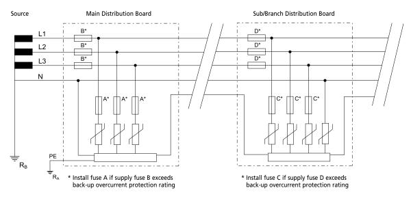
SPDs shown connected L-PE and N-PE. May also be connected L-N and N-PE.
