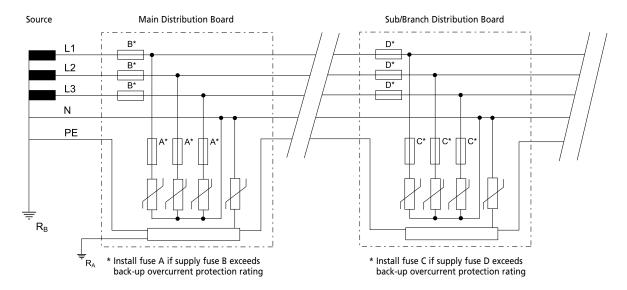
SPDs shown connected L-N and N-PE. May also be connected L-PE and N-PE.
