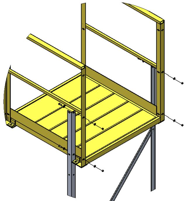
Platform assemblies must not have an unsupported span of over 120" (three Bridges). If a longer crossover is needed, plan Leg Kit locations so the unsupported span is not greater than three bridges.
