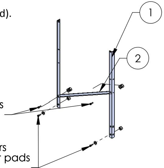
Fasten the (2) Vertical Legs to ladder or platform as shown by torquing (4) 3/8" bolts and nuts and (8) washers (included) to 30Ft-Lbs. Do not face threaded end of the bolt toward the traveled side of the ladder or platform. Do not fully tighten fasteners until all steps are completed.
