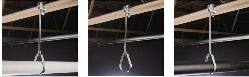
The 115 Standard Duty Loop Hanger is ideal for suspending stationary, non-insulated pipe lines, including CPVC pipes, in fire sprinkler systems. A knurled insert nut helps simplify vertical adjustments and flared edges on the base (1/2" to 4" sizes) help protect pipes from coming into contact with any sharp edges of the hanger.
