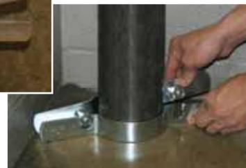
2. Hold bolt in place while aligning clamp
