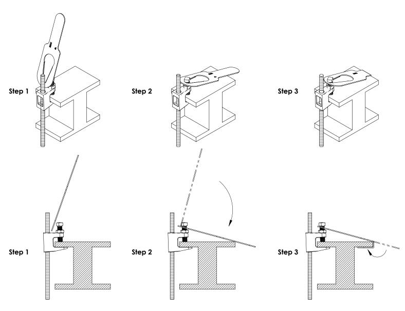
Retaining Strap can be installed on either the set screw or the threaded rod. Retaining Strap can be installed on either the top or the bottom flange.
