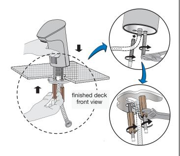
Step 1 Attach faucet to deck (3 hole) Three hole mount with deck plate
