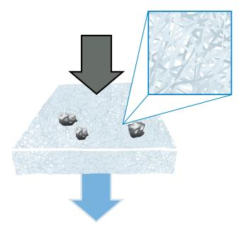
\*Glazed: This process involves putting the felt media through heated rollers to melt back the loose surface fibers to prevent process fluid contamination
