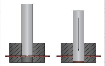
Cut a piece of shim stock to size and place it beneath the block needing shimmed. Use a transfer punch to mark any hole positions. Using a shim stock hole punch set, place the shim stock in the punch block/die set. Maintain consistent pressure on the shim to keep it from moving, remove the transfer punch, install the shim punch, and punch the hole for a perfect fit.
