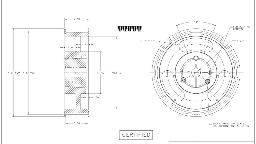
TOOTH TYPE: GT BELT PITCH: 14M PITCH DIA: 14.036 NO. OF TEETH: 80 MATERIAL: GRAY IRON FINISH: 250 v CDATINGS: ANTI-RUST
