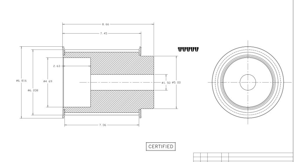
TOOTH TYPE: GT BELT PITCH: 14M PITCH DIA: 6.316 NO. OF TEETH: 36 MATERIAL: DUCTILE IRON
