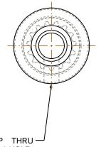
6-40 UNF- 2B TAP THRU = #33 DRILL ( 0.110 )  $\overline{\psi}$  0.200 -( 1 ) HOLE
