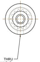
6-40 UNF- 2B TAP THRU - #33 DRILL ( 0.110 )  $\sqrt{\phantom{0}}$  0.200 -( 1 ) HOLE
