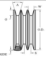
The length shall be measured by placing the belts on two sheaves of equal diameters that have been grooved in accordance with standard specifications and rotated at least three complete turns with the specified tension so that each strand receives half the total tension. The length will be that length obtained by adding the Reference Circumference of one sheave at dimension 'W' to twice the center distance (dimension 'Y').
