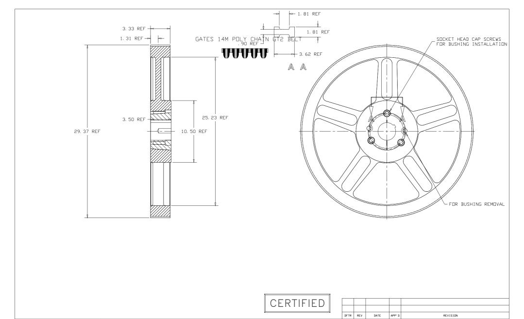
TOOTH TYPE: GT BELT PITCH: 14m PITCH DIA: 29.475 NO. OF TEETH: 168 MATERIAL: GRAY IRON FINISH: 250 v CDATINGS: ANTI-RUST
