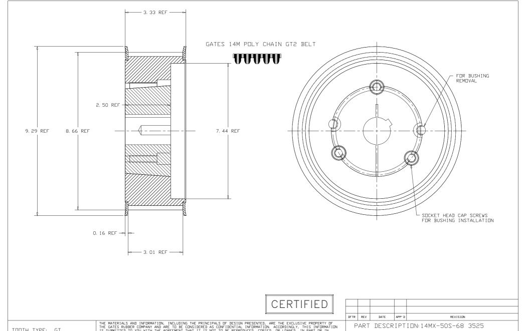
TOOTH TYPE: GT BELT PITCH: 14m PITCH DIA: 8.772 NO. OF TEETH: 50 MATERIAL: DUCTILE IRON
