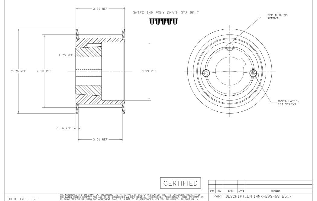
BELT PITCH: 14m PITCH DIA: 5.088 NO. OF TEETH: 29 MATERIAL: GRAY IRON FINISH: 250 v CDATINGS: ANTI-RUST
