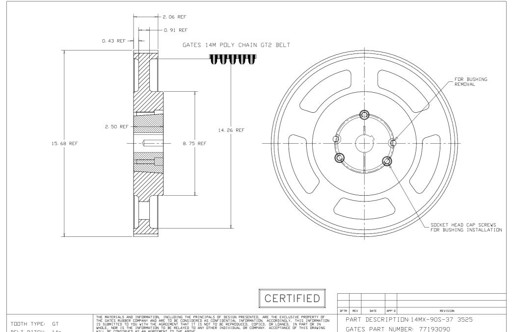
BELT PITCH: 14m PITCH DIA: 15.790 NO. OF TEETH: 90 MATERIAL: GRAY IRON FINISH: 250 v CDATINGS: ANTI-RUST
