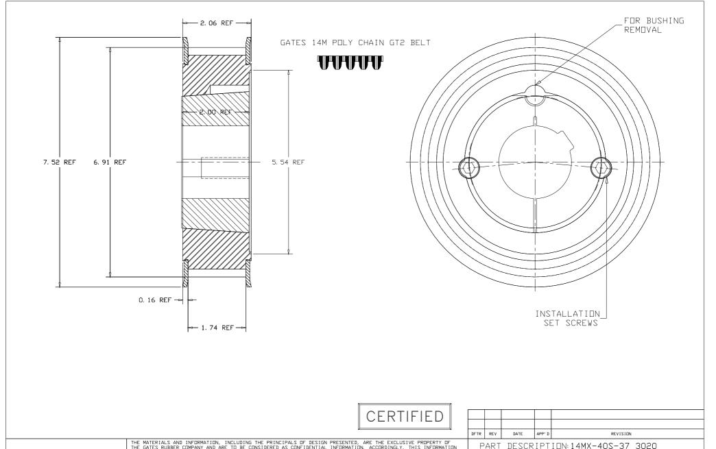
TOOTH TYPE: GTX BELT PITCH: 14m PITCH DIA: 7.018 NO. OF TEETH: 40 MATERIAL: GRAY IRON FINISH: 250 √
