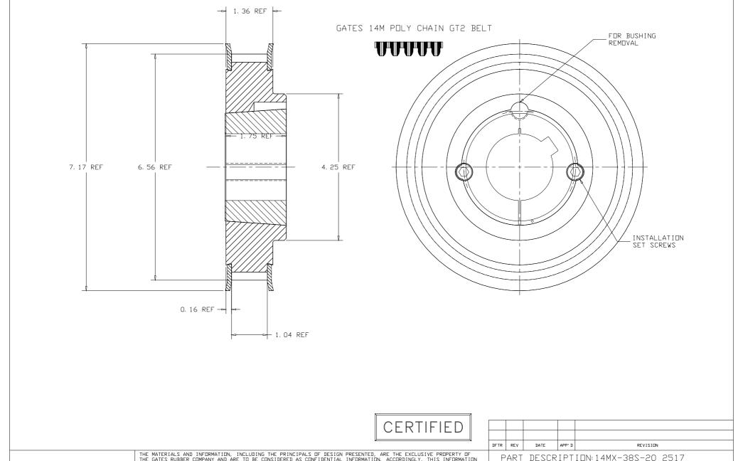
TOOTH TYPE: GT BELT PITCH: 14m PITCH DIA: 6.667 NO. OF TEETH: 38 MATERIAL: GRAY IRON FINISH: 250 v CDATINGS: ANTI-RUST
