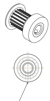
(1) 6-40 UNF 2B TAP THRUTO BORE #33 DRILL ( 0.110 ) THRU TO BORE
