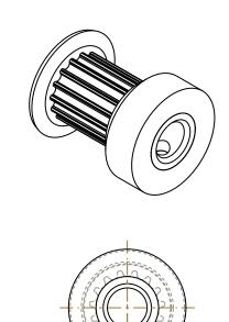
(1) 6-40 UNF 2B TAP THRUTO BORE #33 DRILL ( 0.110 ) THRU TO BORE
