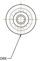
(1) 6-40 UNF 2B TAP THRUTO BORE #33 DRILL ( 0.110 ) THRU TO BORE
