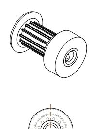
(1) 6-40 UNF 2B TAP THRUTO BORE-#33 DRILL ( 0.110 ) THRU TO BORE
