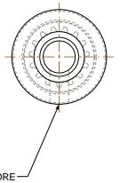
(1) 6-40 UNF 2B TAP THRUTO BORE #33 DRILL ( 0.110 ) THRU TO BORE
