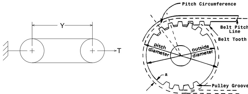
The length shall be measured by placing the belts on two pulleys of equal diameters that have been grooved in accordance with standard specifications and rotated at least three complete turns with the specified tension so that each strand receives half the total tension. The length will be that length obtained by adding the Pitch Circumference of one pulley to twice the center distance (dimension 'Y').
