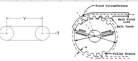
The length shall be measured by placing the belts on two pulleys of equal diameters that have been grooved in accordance with standard specifications and rotated at least three complete turns with the specified tension so that each strand receives half the total tension. The length will be that length obtained by adding the Pitch Circumference of one pulley to twice the center distance (dimension 'Y').
