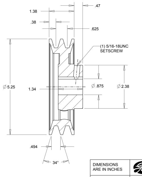
This drawing is a stock power transmission component. Details shown which do not affect drive function may be changed without any notification.
