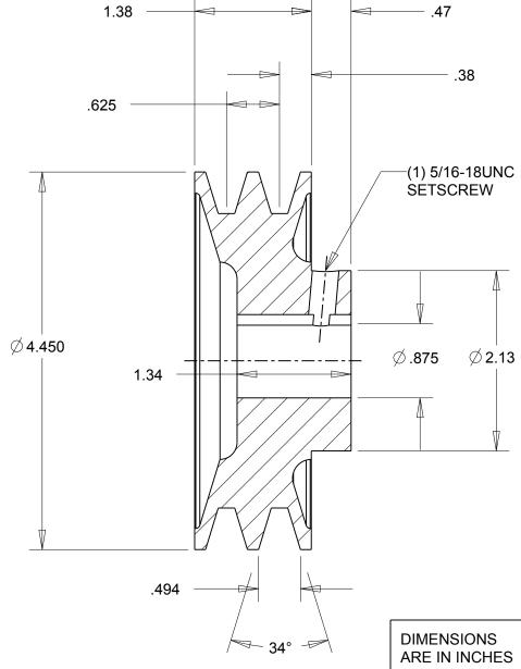
This drawing is a stock power transmission component. Details shown which do not affect
