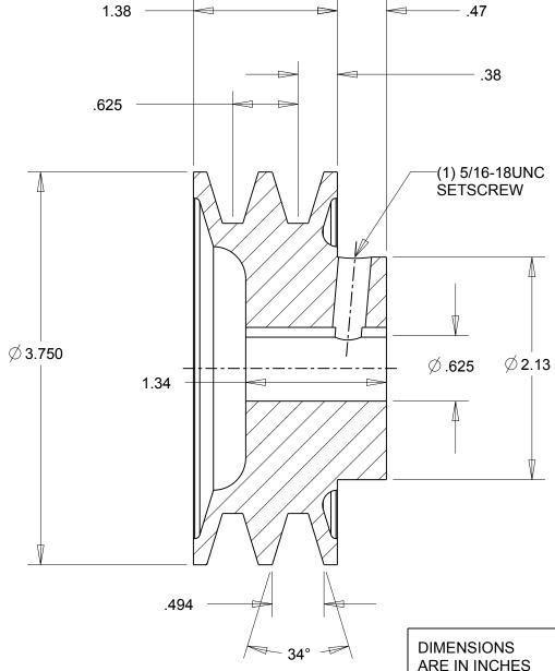
This drawing is a stock power transmission component. Details shown which do not affect
